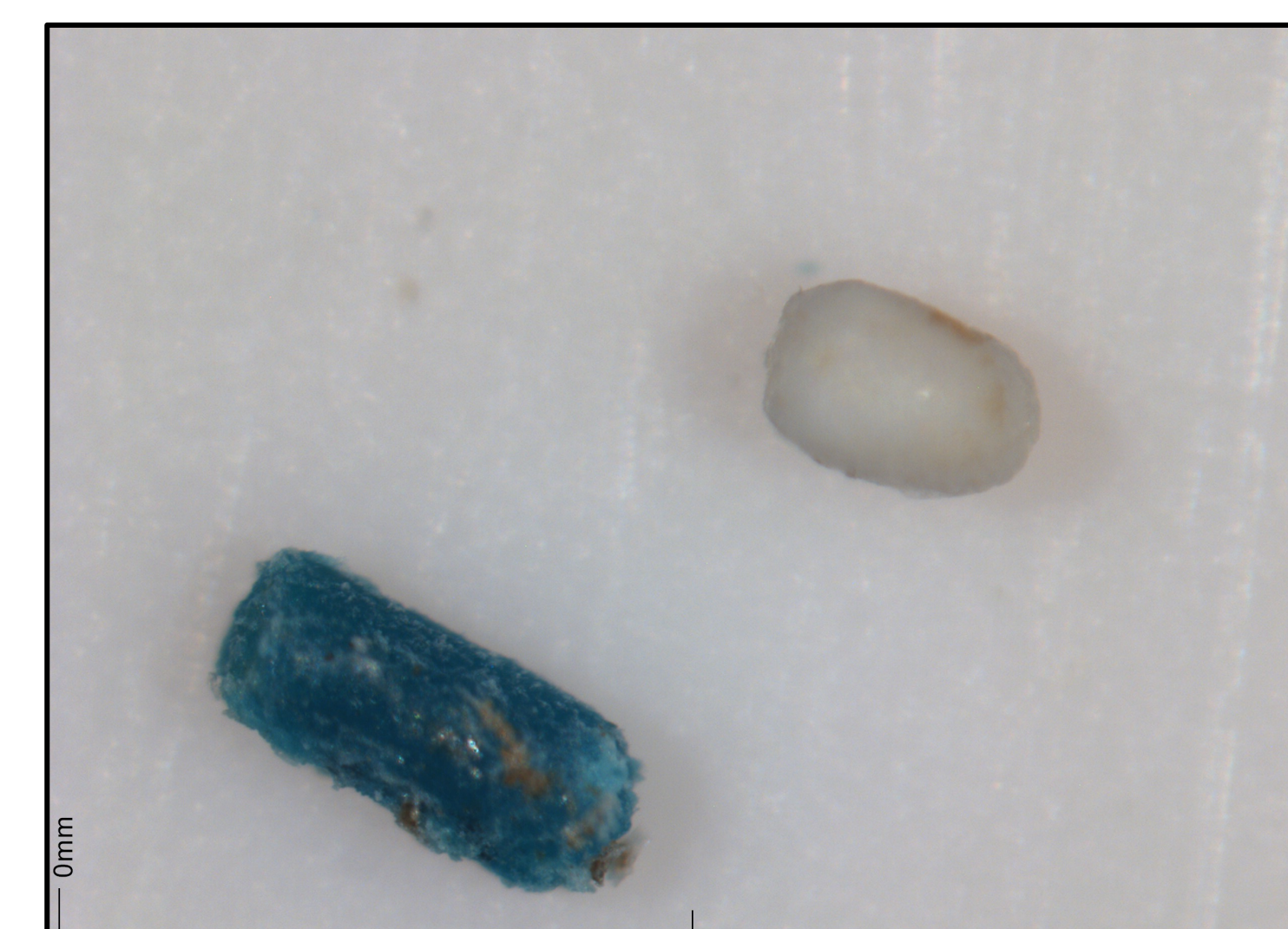
Photo of Site C sample from 10/22/21: 1 fragment and 1 pellet. Field of view = 1.95mm
