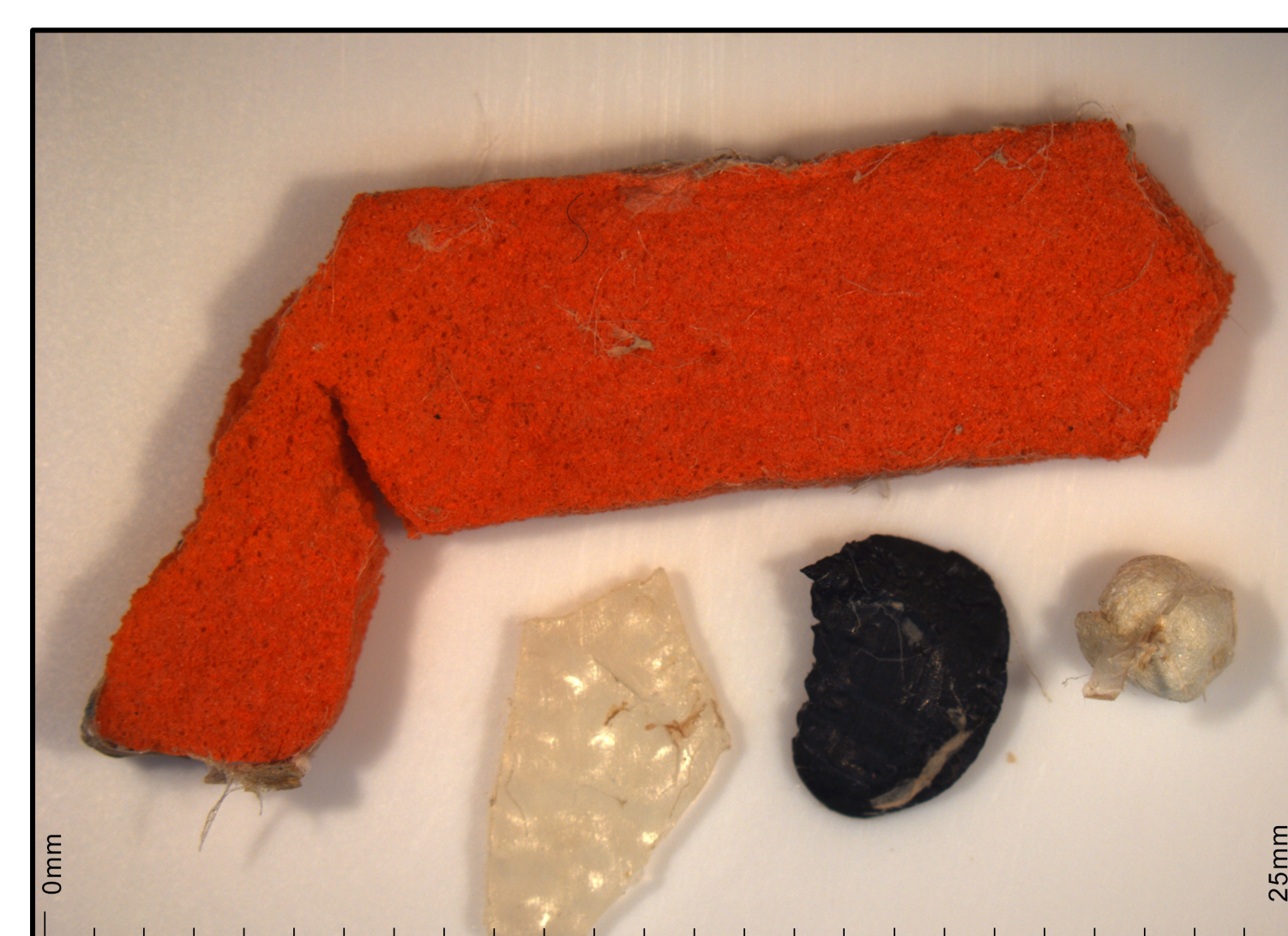
Photo of Site A sample from 9/28/21: foam, fragment, tire particle, and Styrofoam. Field of view = 25mm
