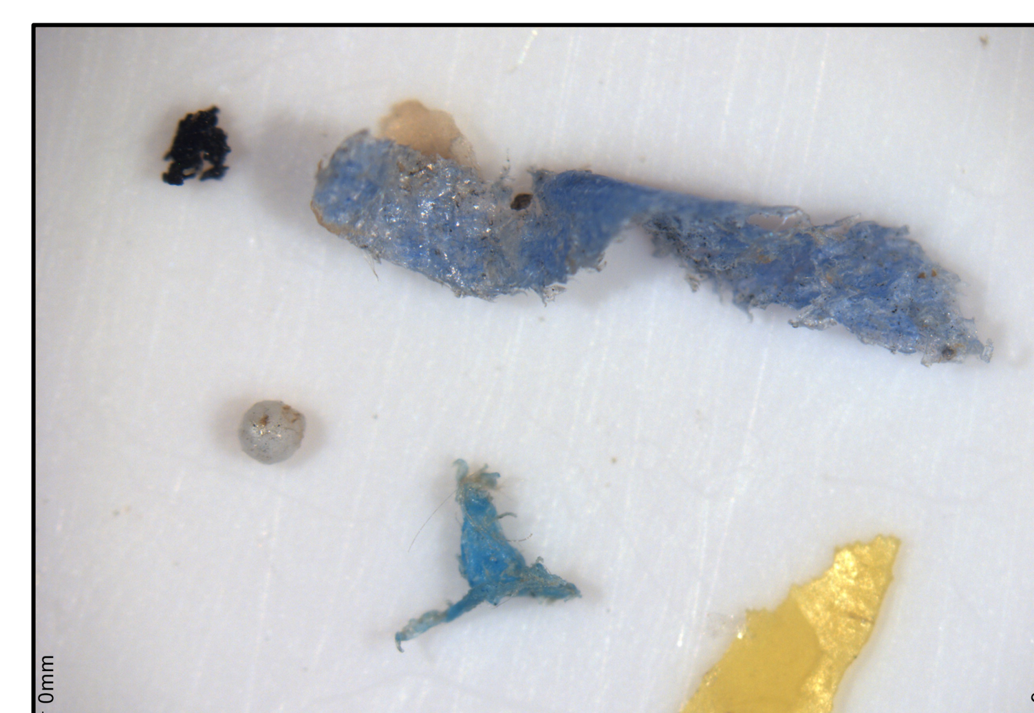
Photo of Site A sample from 10/15/21: 3 fragments, 1 pellet, and 1 tire fragment. Field of view = 9mm
