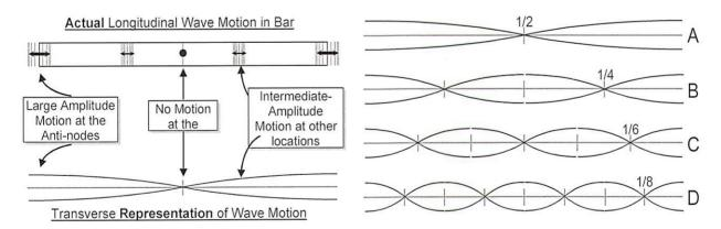
A standing wave in the rod has nodes, or regions where the rod does not vibrate at all, and antinodes, or regions where the rod is vibrating at its maximum. A rod will always have antinodes at its ends. The lower diagram shows the four standing wave patterns that will occur in the singing rods. Each pattern has antinodes at the ends of the rod and equally spaced nodes in between.
