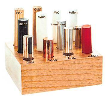
Note: The three white plastics may be difficult to identify. The translucent white plastic is nylon, the bright opaque one is teflon, and the third is PVC.
