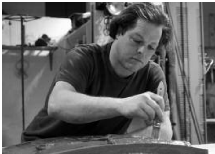
David Huebner brushed the clay models with shellac and a mold release agent before casting them in plaster.
